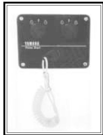
Engine Stop Switch
