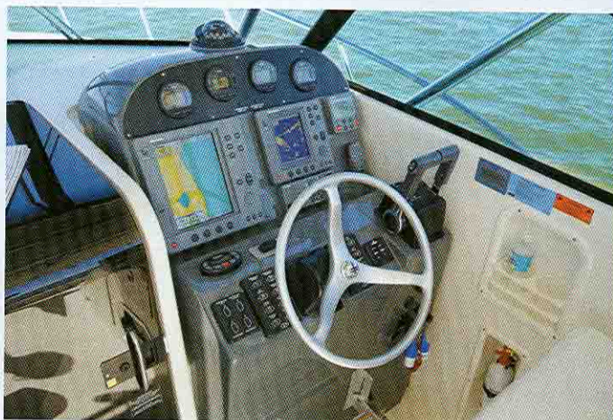
The helm offers all the information a skipper needs in a tight and efficient layout. Important instruments and displays are within the line of sight for quick reference.
